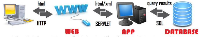
Fig. 1: Three Tiers of Web, Application and Database Servers
